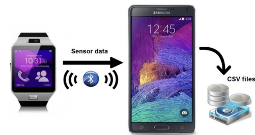
Figure 2: Data collection methodology for wearable device sensor data
